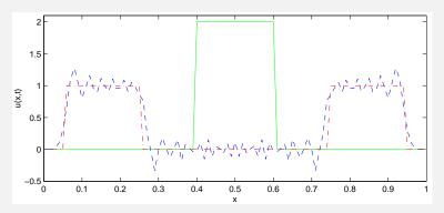
**Observations:** • Strong oscillations (as in the leapfrog scheme for (AE) [there is no damping (artificial viscosity)]
