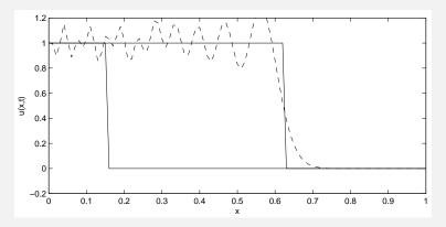
Observation: Strong oscillations (due to missing artificial viscosity)
