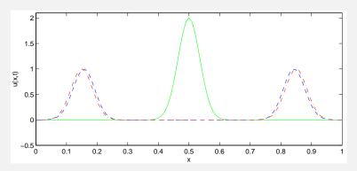
**Observations:** • Initial pulse splits into two smaller pulses travelling into opposite directions.
