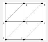
**Consider**  $\triangle 012$ :  $\iint_{\Delta 012} \left(0^2 + \frac{1}{h^2}\right) dx dy = \frac{1}{2}$  and the same from  $\triangle 023$ ,  $\triangle 045$ , and  $\triangle 056$  by symmetry.
