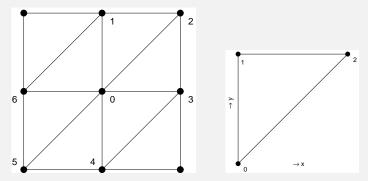
**Consider**  $\triangle 012$ : For equal sides *h*. Without loss of generality, we can move the origin to node 0.
